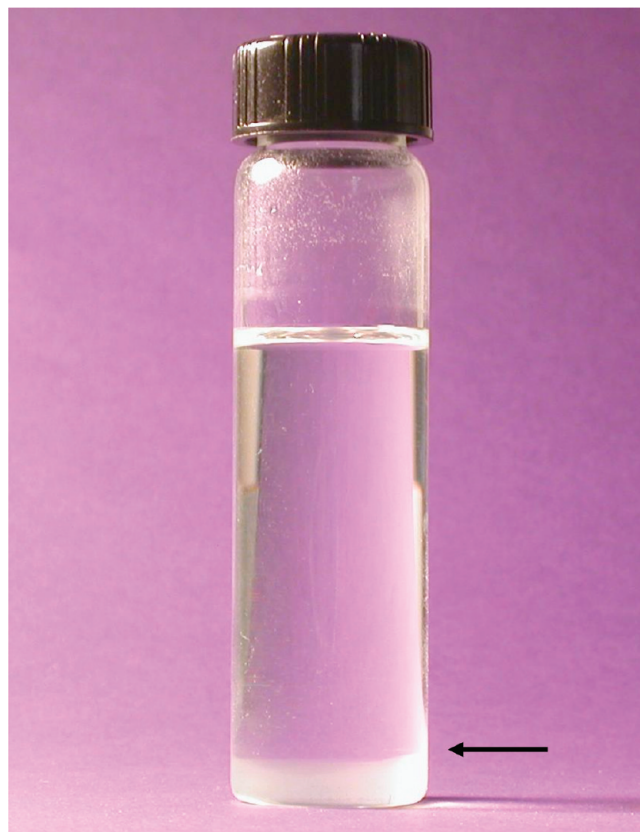
Figure 6. Photograph illustrating uneven distribution of fumed silica (CAB-O-SIL M-5) to the bottom NBR phase of SBR/NBR 90/10 blend in toluene solution.
